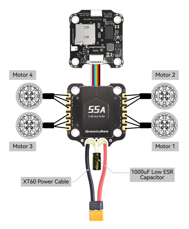
**Note1**: In order to prevent the stack from being burnt out by voltage spikes on powering up, it is strongly recommended to use the Low ESR capacitor in the package.
